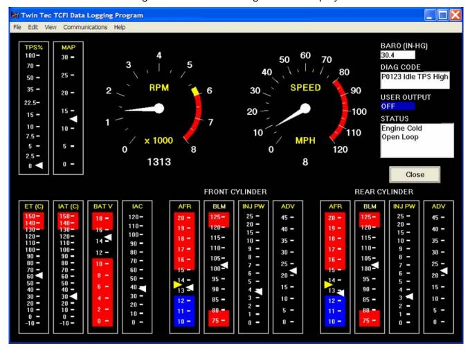
Figure 1 – Real Time Engine Data Display
